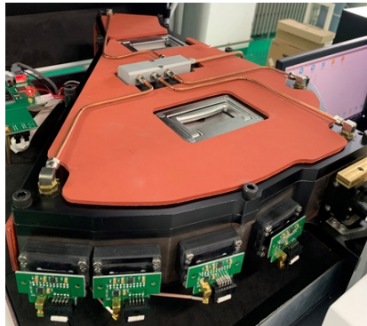
Spectrometer Layout with CCD and Channel Electronics.
