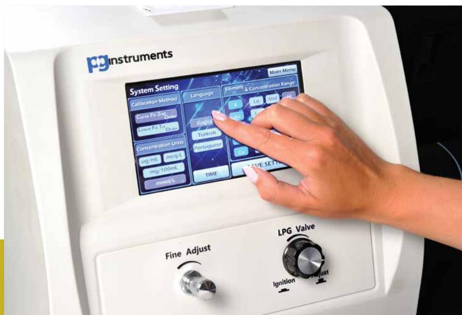
Selection of analytical parameters using touch screen.
