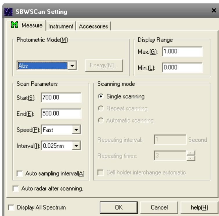
Figure 8-1 Bandwidth scanning parameters setting
