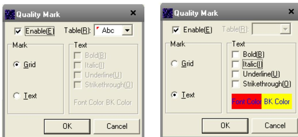
Figure 4-4 Quality Mark Marking Grid (Left) Marking Text(Right)
