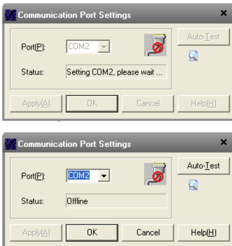
Figure 2-14 Communication Port Setting Window - Online (Up); Offline (Down)
