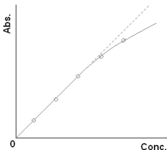
Figure 6-4 Nonlinear Calibration Curve
