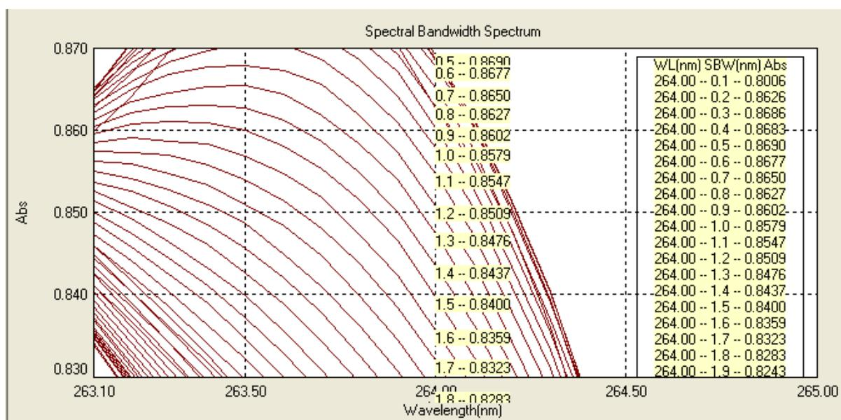
Figure 8-4 Spectral Bandwidth scanning spectrum of Benzylpenicillin potassium
