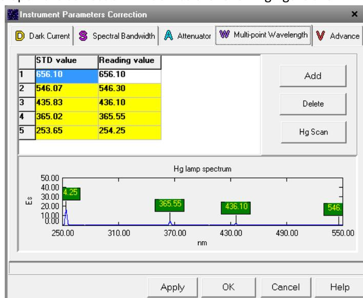
Figure 3-6 Wavelength Correction with multi-point
